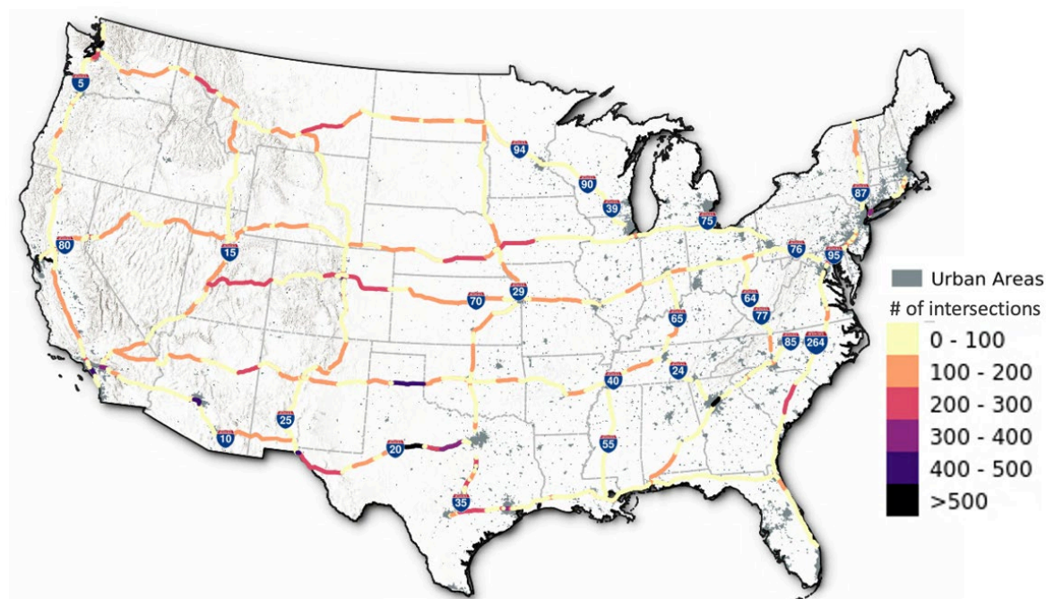
Figure V-12. Highway segments and the count of intersections with other roads, natural gas pipelines, and railroads.
